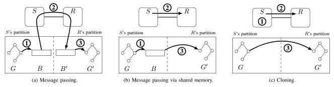
Fig. 2: Schematic comparison of approaches to transfer an object graph G from sending core S to receiving core R. Temporary buffers are denoted by B, B'; and G' is the resulting copy of G.
