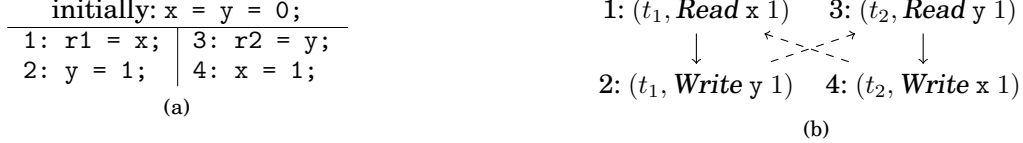
Fig. 3: Program from Fig. 1a in simpler syntax (a) and its JMM execution for the result r1 == r2 == 1 (b).
