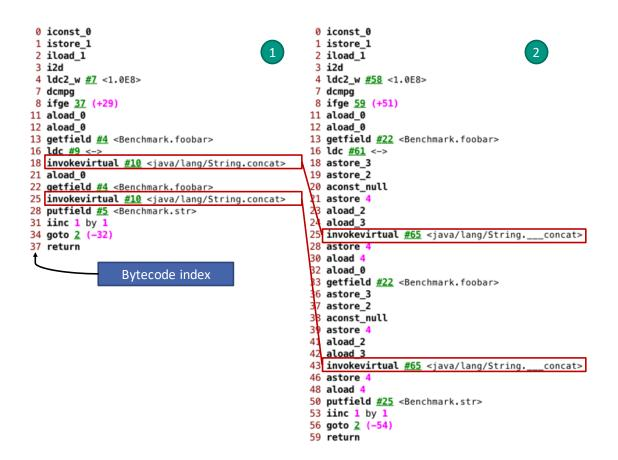
Figure 5.5.: The SelectiveTaintingInstrumenter modifies the call instructions considered safe by the JOANA-Adapter in the bytecode as the classfile gets loaded into them JVM.
